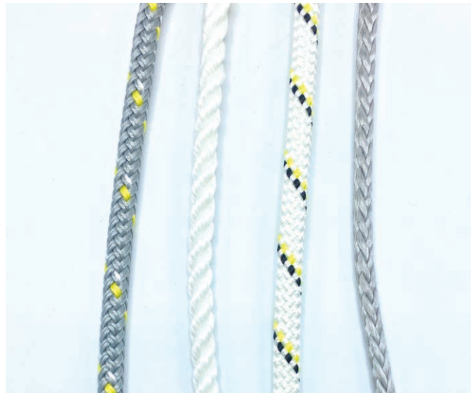
ABOVE LEFT TO RIGHT—1. Raid Braid polyester double-braid from Duckworks. 2. Typical 3-strand line. 3. Marlow's Excel Racing with Dyneema core. 4. Samson's Amsteel Blue 12-strand Spectra.
